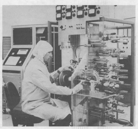
machine that I modified. It still has the manufacturer's nameplate on it — Hilton Industries — but that's about the only part left of the original machine. We completely rebuilt it to get the precision windings we needed."
